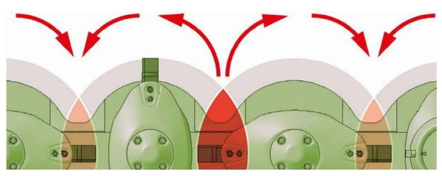
Figure 1: Top view of the overlapping zones of the KRONE EasyCut cutterbar; red arrows show the direction of rotation of the discs, orange zone = overlapping area where the blades move backward and red area = overlapping area where the blades move forward (MASCHINENFABRIK BERNHARD KRONE GMBH & Co. KG 2022)
